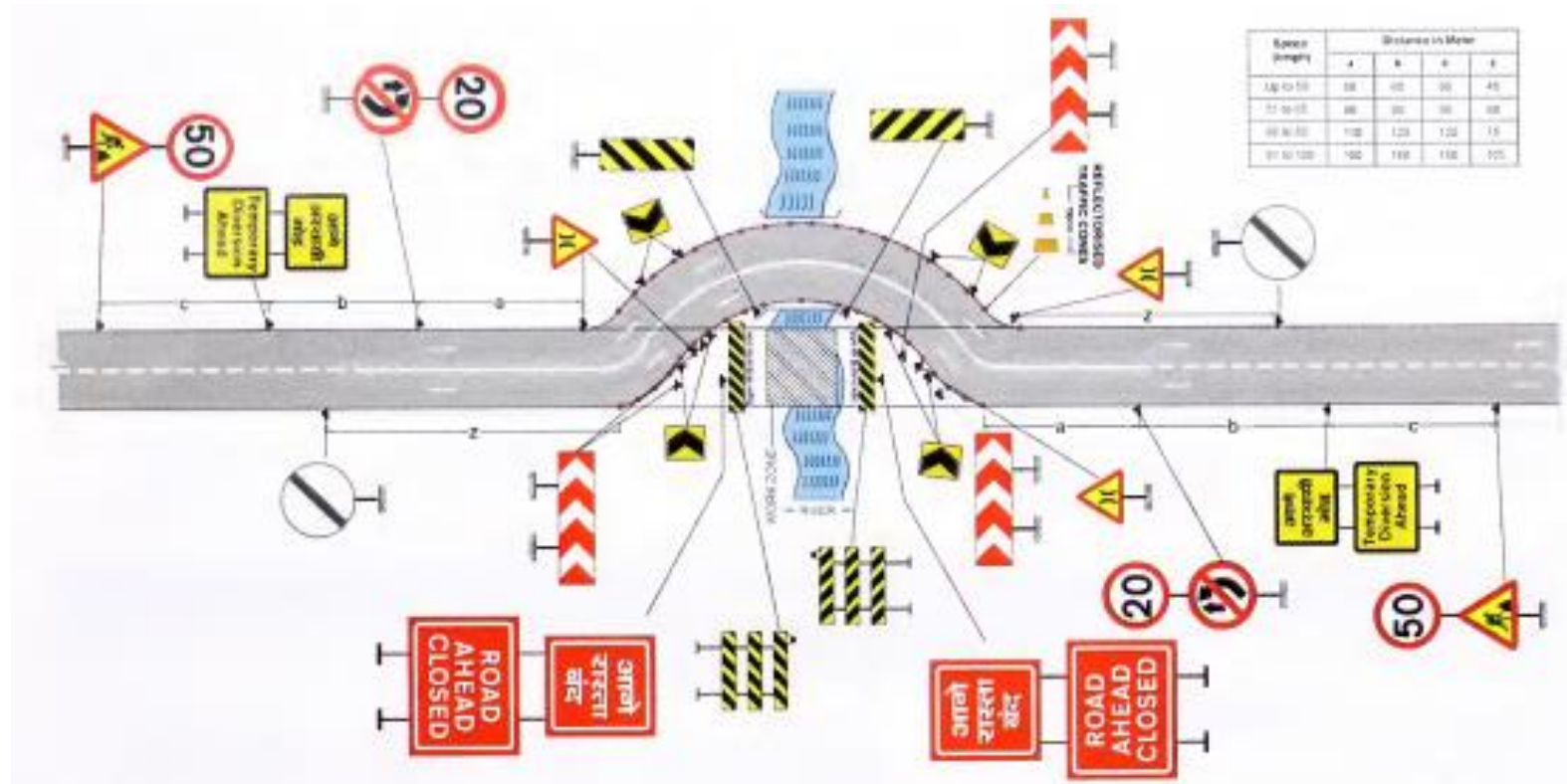
Figure-5 Temporary Diversion for Reconstruction of CD works
